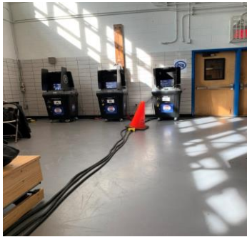
Image description - cables across the floor leading to scanners, a tripping hazard and a barrier for people using wheelchairs.
